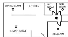
Figure 1: Locations for placing Smoke Alarms for single residence with only one sleeping area.
