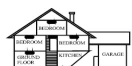
Figure 3: Locations for placing Smoke Alarms for a multi-floor residence
