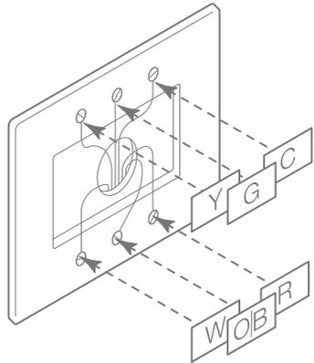
**CAUTION:** Wiring can vary for each manufacturer. Label all wiring before removing it from the existing thermostat.
